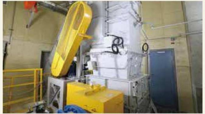
**回転式破碎機** Roller crusher
